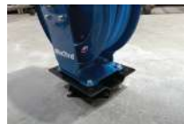
Attach top plate and reel to the bottom plate.
