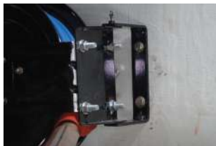
Place the reel onto the mounted base plate.
