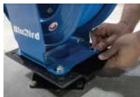
Attach top plate to the reel.
