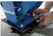
Attach top plate to the reel.
