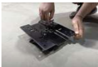
Detach top plate from the bottom plate.
