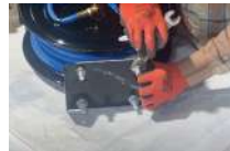
Attach the reel to the swivel arm and secure it with bolts.
