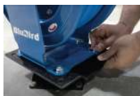
Attach top plate to the reel.
