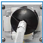
Four rollers reduce hose wear
